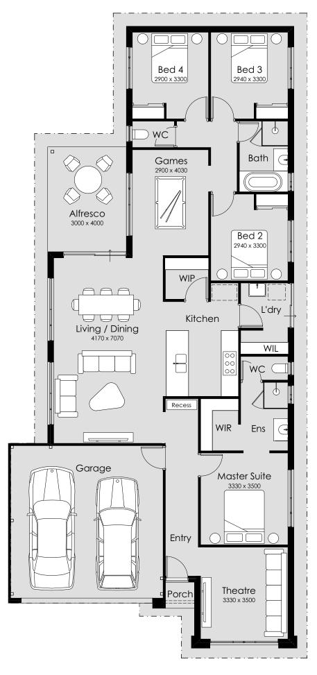
OVERALL WIDTH- 11.01m OVERALL LENGTH- 23.71m MIN BLOCK WIDTH- 12.50m MIN BLOCK LENGTH- 30m TOTAL AREA- 208.21m<sup>2</sup>
